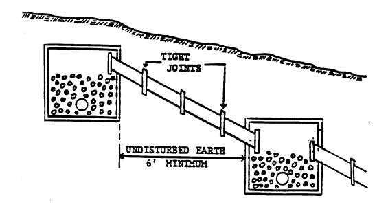
\*\* Differing ground slopes over subsurface disposal fields may require use of various combinations of fittings.
